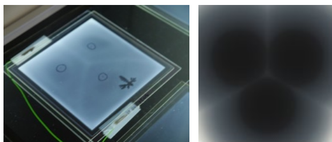
Figure 1. Experimental photograph of ODF mura (left) model of deformation to the director structure (right).
