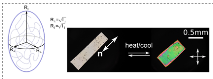
Diagram of the polymer conformation of an LCE in the nematic state (left). The shape change seen on heating a film of nematic LCE, the change in order causing a change in polymer conformation (right). Taken from 2.
